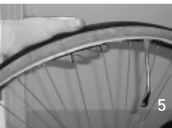
The tyre should remain sitting on one side of the rim. Grab the inner tube at the valve hole, push the valve up through the rim and pull the valve out from the tyre. Pull the rest of the inner tube out.
