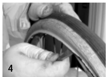
Take the middle lever out and repeat the process a few times. Once about a third of the tyre is hooked over the rim, the remainder will come off more easily.
