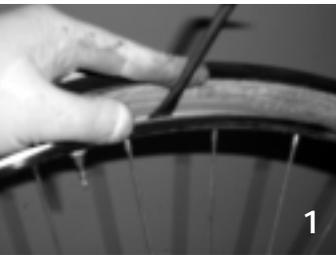
Fit 2 or 3 tyre levers into the rim about 2cm apart and pull them back, levering one side of the tyre out and over the side of the rim. Take care you are not pinching the tube while you lever the tyre out.
